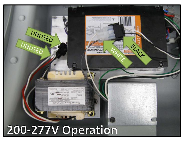
B) For 200-277V Operation: Connect the White Wire Chamber Connector to the Black Ballast Connector. (You will leave the transformer connectors disconnected)
