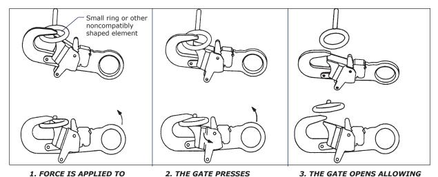
**2.2 MAKING CONNECTIONS:** Only use self-locking snap hooks and carabiners with this equipment. Only use connectors that are suitable to each application. Ensure all connections are compatible in size, shape and strength. Do not use equipment that is not compatible. Ensure all connectors are fully closed and locked.
