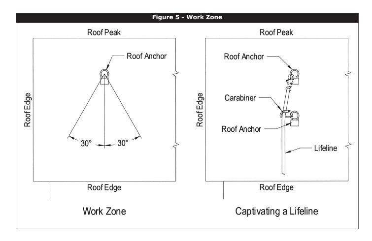
the anchorage point. It is acceptable to captivate a lifeline to an anchorage close to the work area with a carabiner. Do not captivate the lifeline of a self retracting lifeline.
